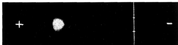
Paper electrophoresis of cysteinyl-glycinase. 0.04 M THAM-HCl buffer, pH 8.2, + 0.0005 M MnCl 2 ; 400 V during 3 h at room temperature on Whatman N 54. The cysteinyl-glycinase activity is shown by the green-grey spot (white in the figure) against a pink background (black in the figure).
